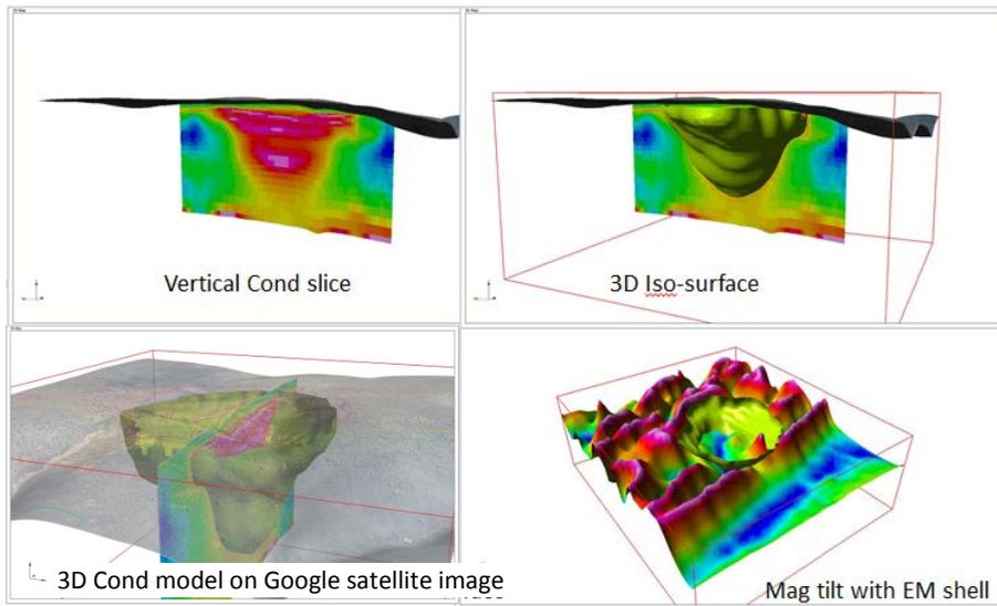
Figure 5: 3D views of conductivity inversion results and data.
