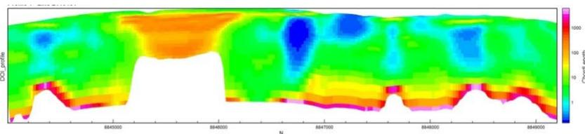
Figure 3: Conductivity-Depth Image (CDI) showing thick conductive crater in-fill.
