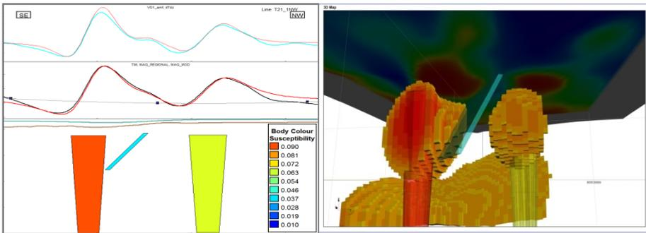
Figure 6: Examples of magnetic parameterized body profile modeling (left) and 3D magnetic susceptibility inversion (John Paine-UBC) results (right).
