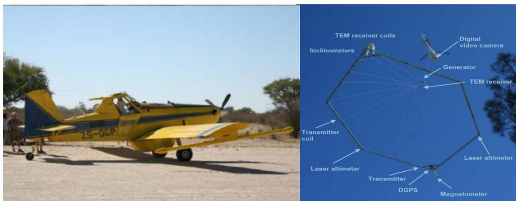
Figure 1: Xcalibur's ultra-high resolution Xtract airborne magnetic system (left) and SkyTEM helicopter-borne EM system with instrument positions shown (right).
