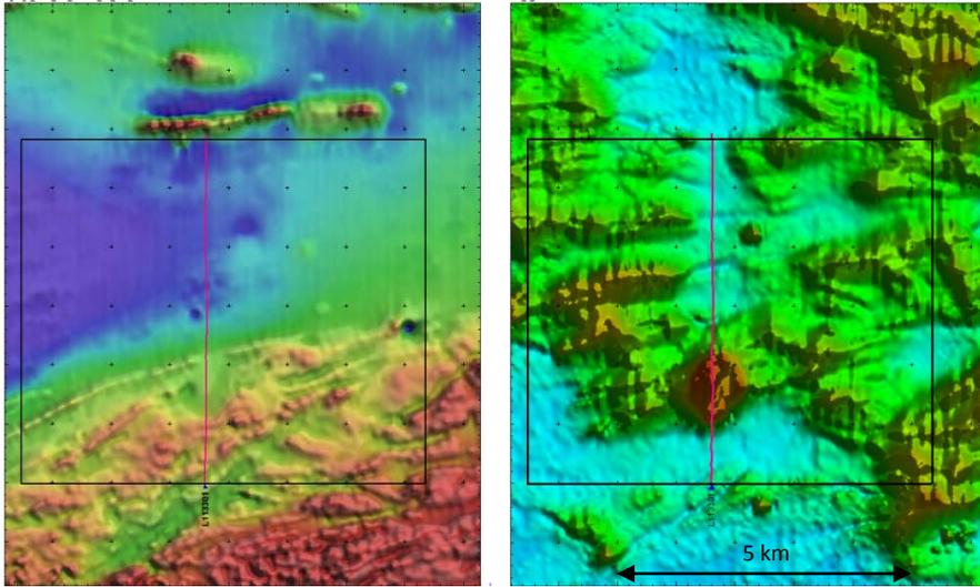
Figure 4. Map view of a number of kimberlite targets with different EM and magnetic signatures. Magnetic RTP grid (left) and EM intermediate channel grid (right).
