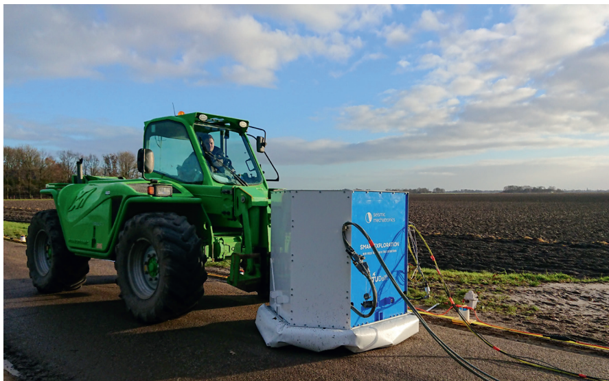
Figure 1 E-Vib validation at a geologically and geophysically known site in the Netherlands (December, 2018).
