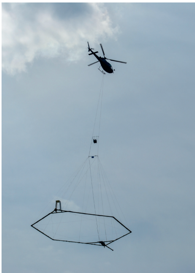
Figure 1 The SkyTEM system was flown for the validation survey at the Blötberget Mine Site, Ludvika, Sweden.
