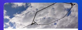
The redeveloped suspended receiver coil system offers a five-fold or more reduction in late time noise levels.
