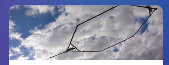
The redeveloped suspended receiver coil system offers a five-fold or more reduction in late time noise levels.
