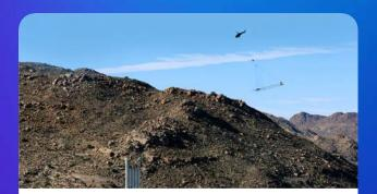
The re-engineered receiver coil system offers a five-fold or more reduction in late time noise levels for greater resolution at depth.
