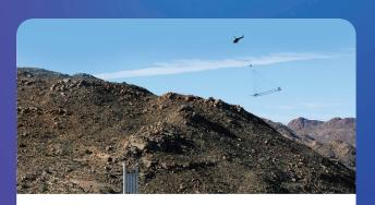
The re-engineered receiver coil system offers a five-fold or more reduction in late time noise levels for greater resolution at depth.
