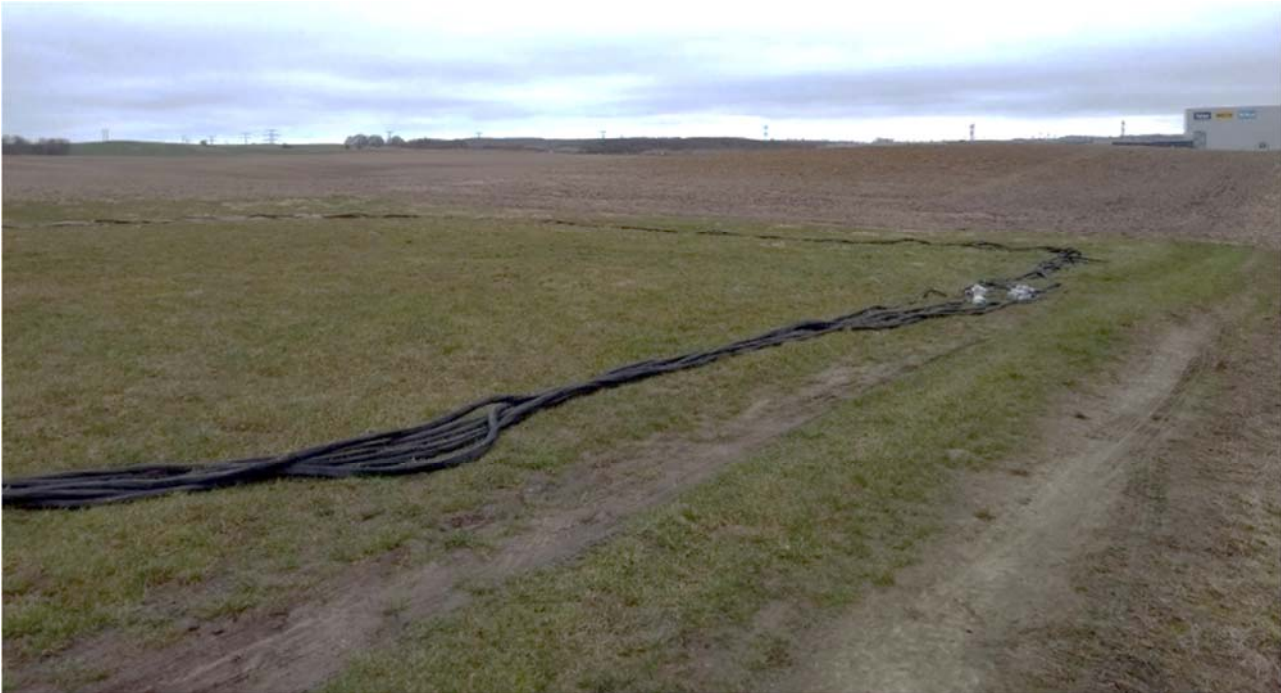
Figure 6: A B-field target consisting of a 521 m 2 wire loop (black cable bundle) was employed for testing the B-field measurements.
