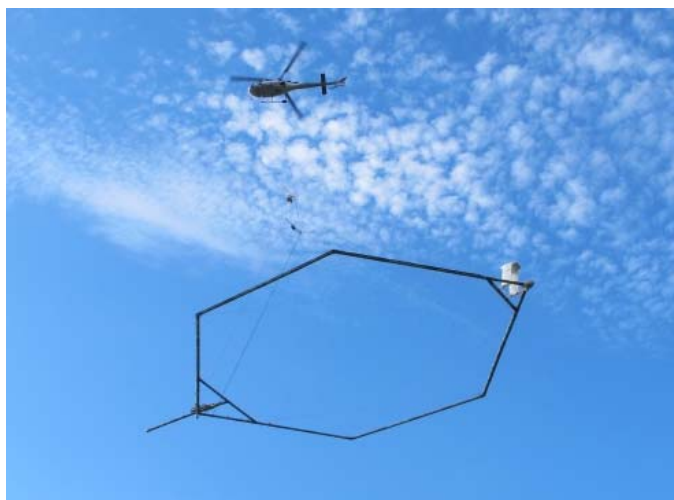
Figure 1: The SkyTEM312 HP system
