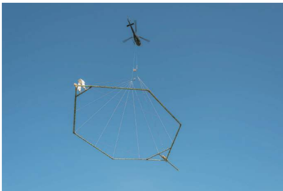
Figure 2: The SkyTEM312 Fast system in operation.
