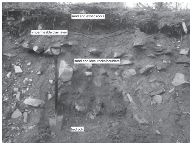
Fig. 1. Typical profile through the glacial till of northern Finland. This till layer is usually 0–10 m thick around the Kevitsa mine site.
