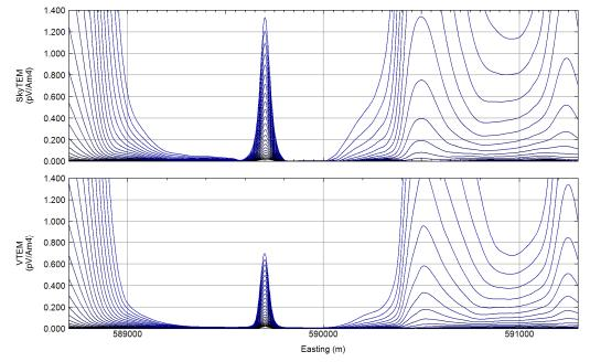
Figure 4: Line 20030, gates 12-35 (see Table 1) for the SkyTEM<sup>508</sup> system (top panel) and the VTEM system (bottom panel).
