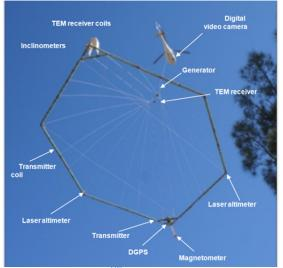
Figure 1: The SkyTEM <sup>508</sup> system at a glance
