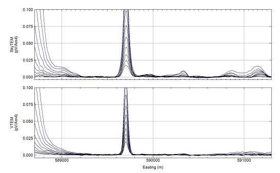
Figure 5: Line 20030, gates 26-35 (see Table 1) for the SkyTEM<sup>508</sup> system (top panel) and the VTEM system (bottom panel)...
