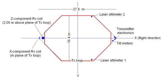
Figure 2 SkyTEM transmitter-receiver geometry for 314 m<sup>2</sup> loop.
