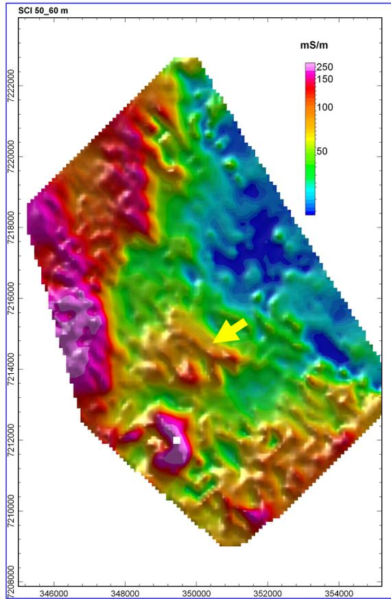
Figure 6 50-60 m SCI depth slice. The arrow indicates the anomalous conductors interpreted as carbonaceous palaeochannels within the Moogooloo Sandstone. Thick Coyrie and Billidee Fm cover is present in the NW of the area.
