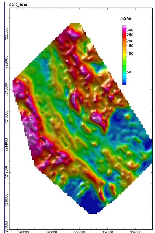
**Figure 5** 0-10 m SCI depth slice. The moderately-conductive zone trending NW through the centre of the area is the modern valley of the Gascoyne River. Highly conductive areas in the NE and NW correspond to outcrop/subcrop of the Coyrie and Billidee Formations. Resistive zones in the SW and SE correspond respectively to Callytharra Fm Limestones and Moogooloo Sandstone.
