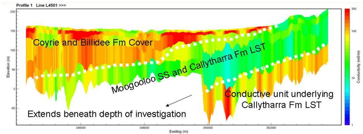
**Figure 6** LCI conductivity cross-section from Line 4501 (Figure 4).
