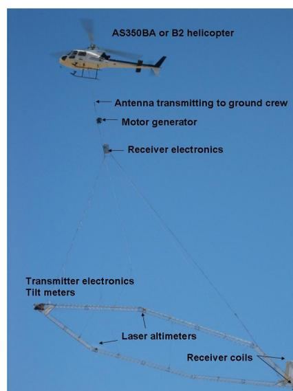
**Figure 1. SkyTEM system in operation in Australia, October 2006 (314 m<sup>2</sup> Tx loop).**
