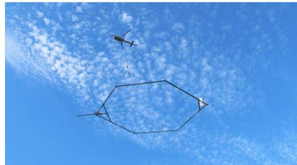
Figure 1 SkyTEM system in flight
