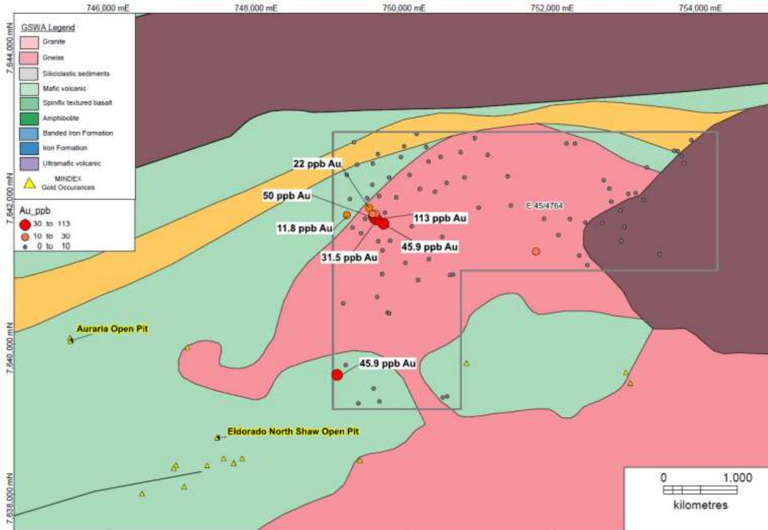
Figure 2. Stream sediment sampling at the Bonnie Scot project E45/4764.
