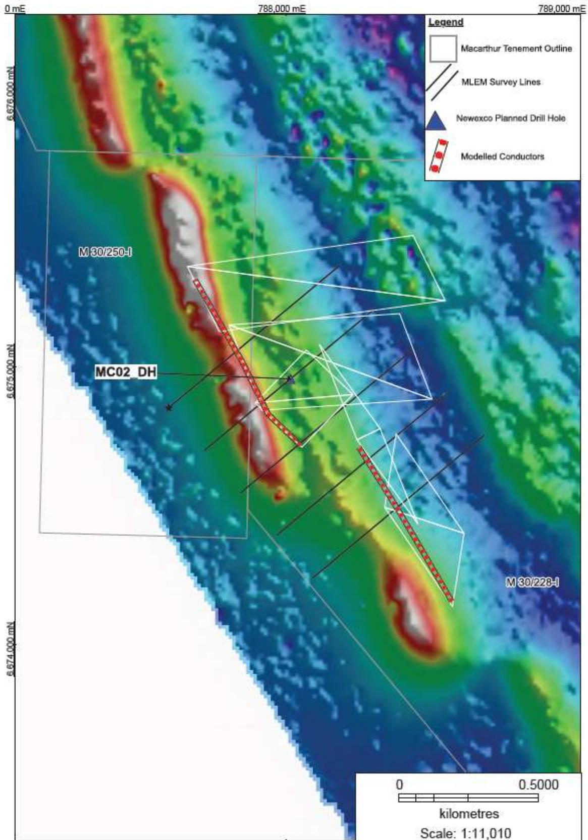
Figure 3. MLEM survey at Moonshine showing modelled conductors. Background image shows magnetic anomalies. Planned drill hole MC02\_DH location.
