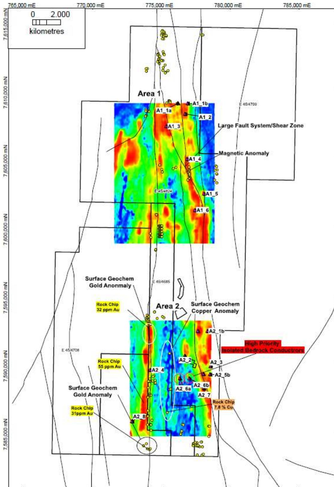
Figure 1. Hillside SkyTEM survey flowchart at 150 m line spacing showing conductors and geochemical anomalies.
