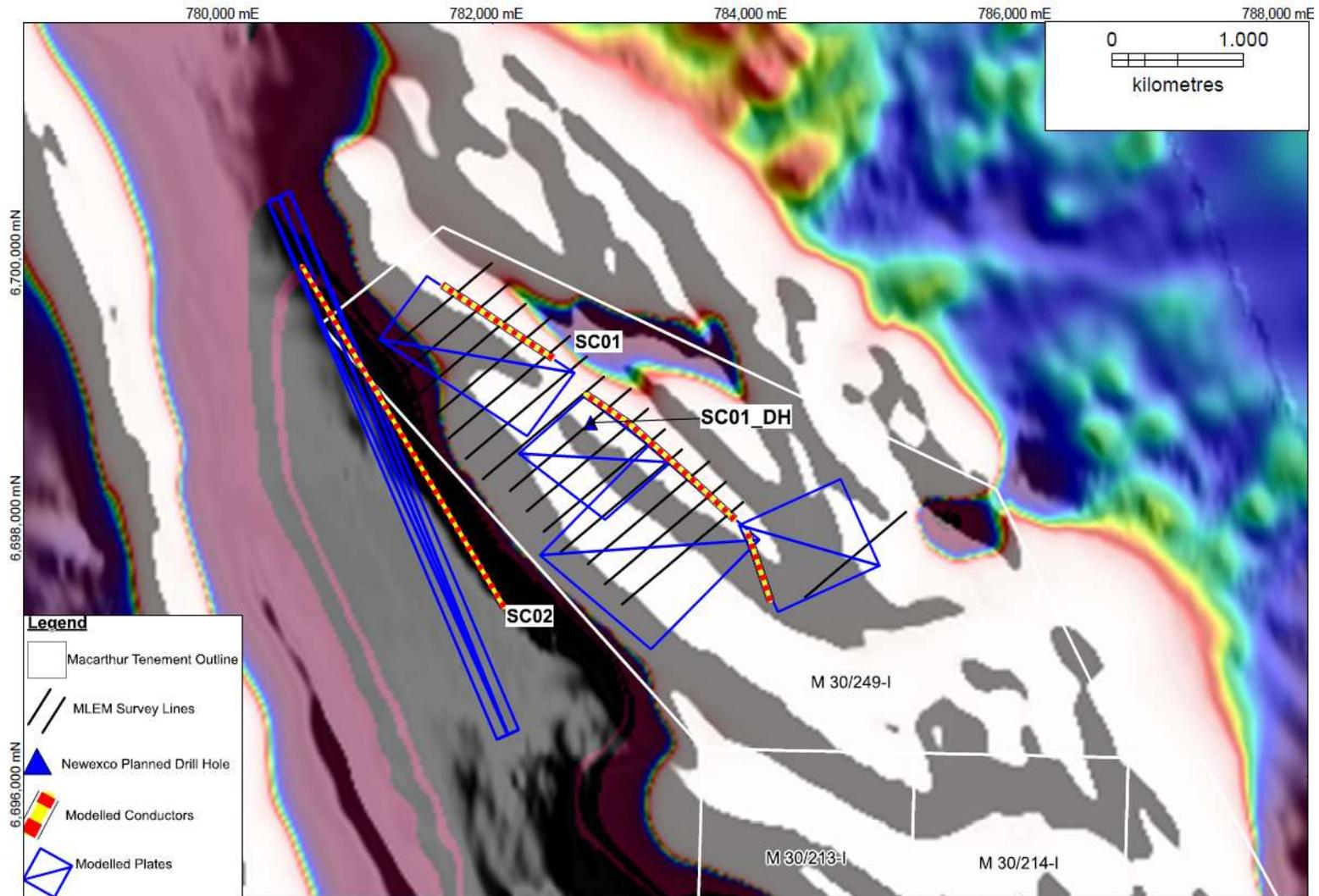
Figure 4. MLEM Survey at Snark showing modelled conductors. Background shows Total Magnetic Intensity anomalies. Planned drill hole SC01\_DH location
