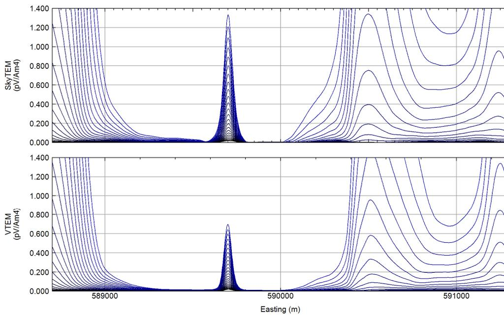
Figure 4: Line 20030, gates 12-35 (see Table 1) for the SkyTEM<sup>508</sup> system (top panel) and the VTEM system (bottom panel).
