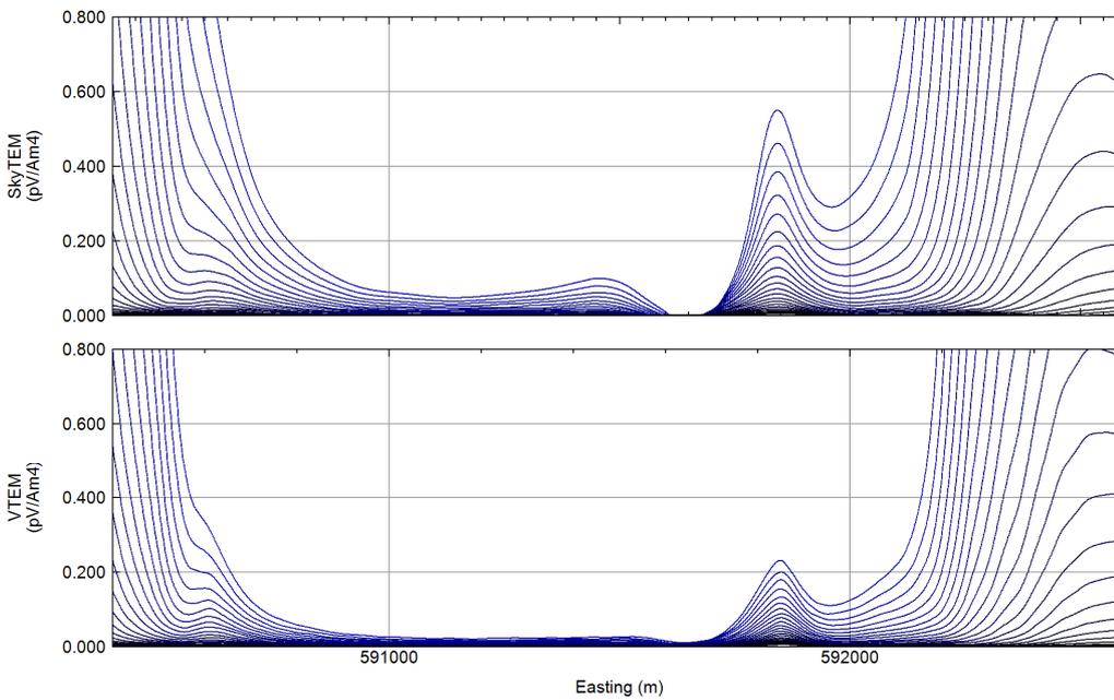
Figure 2: Line 20010, gates 12-35 (see Table 1) for the SkyTEM<sup>508</sup> system (top panel) and the VTEM system (bottom panel)
