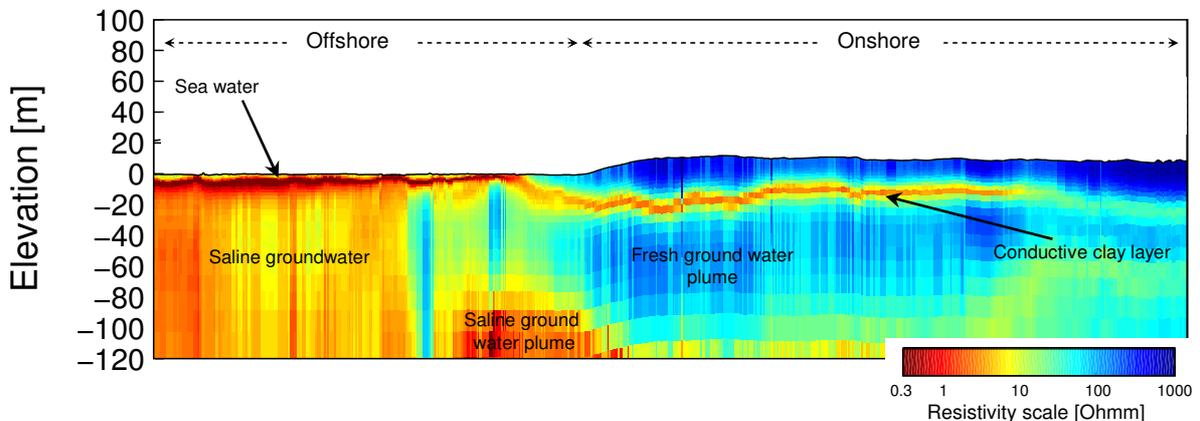
Multi-layer fast approximate inversion of the two lines perpendicular to the coast line. Red colours indicate low resistivity (saline groundwater) and blue colours indicate high resistivity (fresh groundwater).
